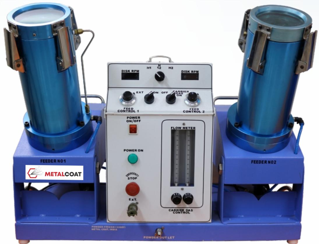
The **MPF 3350 Twin Powder Feeder** is specifically designed for thermal spray coatings. Its small size makes it a portable powder feeder, which can be carried to site for job work. The unit is controlled to extremely precise and repeatable powder feed rates. The powder hopper (canister) is mounted on a
